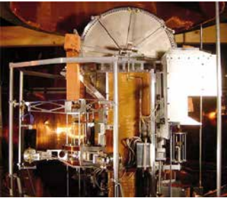
Fig. 4. Balanza del Watt del National Institute of Standards and Technology (NIST), Boulder, Colorado, EUA.
